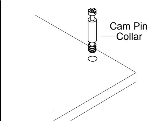
The Cam Pin is inserted into the flat side of a board, it is important that: The cam pin is kept vertical and is not put in on an angle. Cam pin is to be inserted up to collar Too far and it wont catch the Cam Lock (Do Not Overtighten) Not enough and the resulting product will not be stable.
