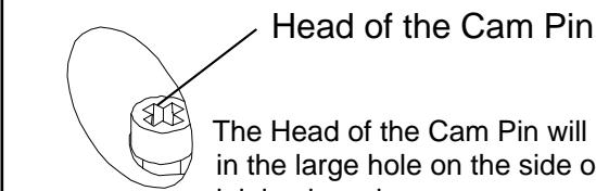
The Head of the Cam Pin will be visible in the large hole on the side of the joining board.
