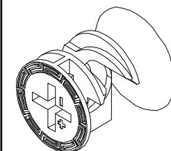
Notice the Cam Lock has a "C" Shaped Back. An arrow or +/- signs on the front indicate the open section on the back of the Cam Pin.
